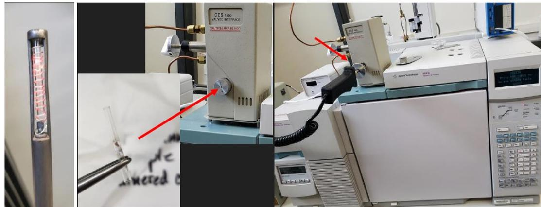
**Fig. 9 (Left) |** A quartz tube with a platinum coil being heated to clean it before loading the sample.
