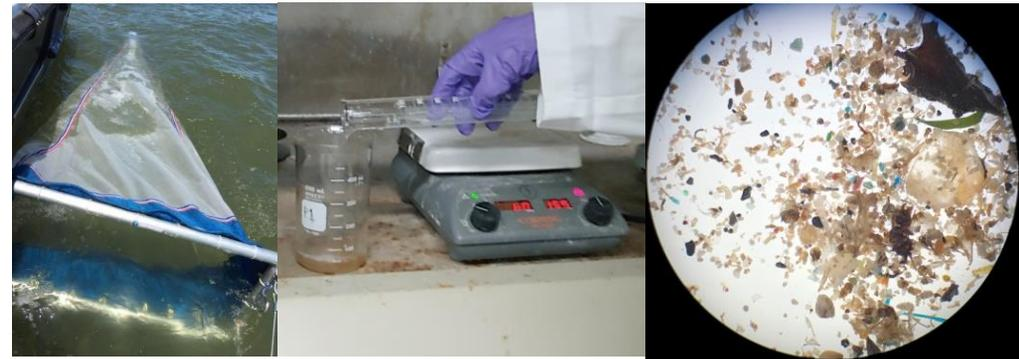
Fig. 2 (Left) | Neuston net during microplastic sample collection.
