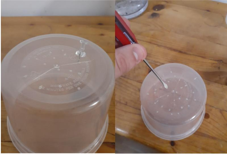
4. Assemble Filter Media (example uses paper towel, sand and tissue paper layers. Remember to try experimenting with your own types of filter media!)
