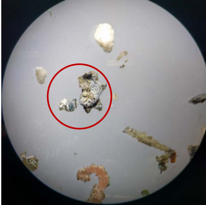
Fig.7. Clusters or amalgamated pieces of microplastics: Many pieces of microplastics are sometimes held together by another microplastic piece. In this case each identifiable microplastic will be counted individually.
