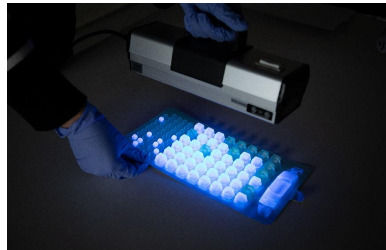
Fig. 2 (below) | One Enterolert* Quanti-tray* with high levels of Enterococcus contamination (blue fluorescence)
