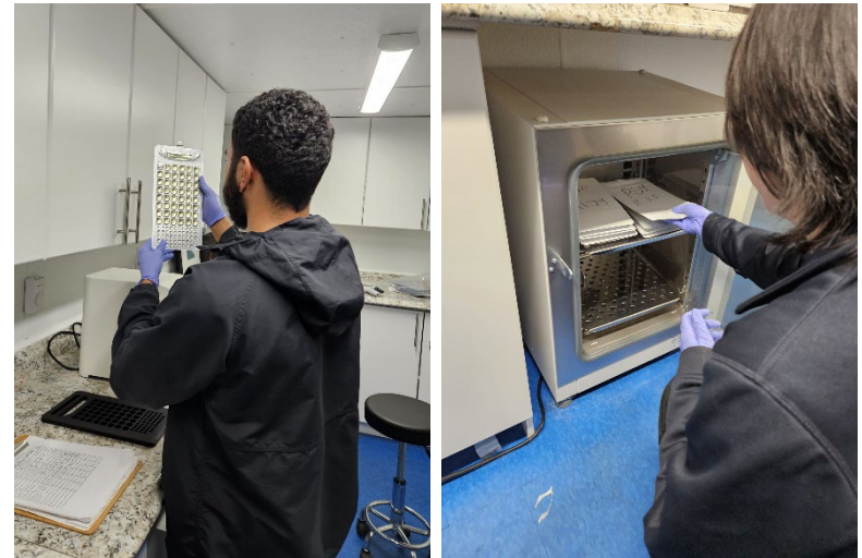
Fig. 1 | Filling (left) and incubation (right) of an Enterolert* Quanti-tray*
