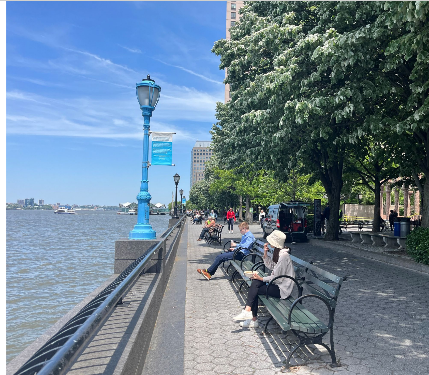
Blue lampposts along the esplanade illustrate the elevation of storm surge for a projected 2050's 100-year storm, including 2.5 feet of sea level rise. This one at Rector Place is approximately 10.5 feet above the Esplanade
