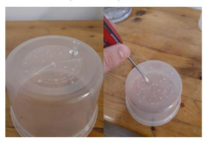
4. Assemble Filter Media (example uses paper towel, sand and tissue paper layers. Remember to try experimenting with your own types of filter media!)
